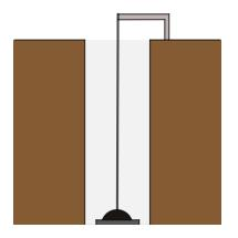
Put the origin at the location of the drill with +y-axis oriented upwards. We consider the drill and chain separately. For the drill, this is a simple matter since the weight of the drill is constant and it is moved the 45 m to the surface:
