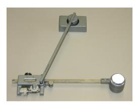
The planimeter consists of a two-bar linkage. At one end there is a pointer which is used to trace a closed curve, while the other arm allows the free movement of the device—though the base of the device remains fixed. The planimeter keeps track of the distance that a wheel fixed in place at the pointer rolls.<sup>2</sup> The planimeter then applies this information, using Vector Calculus, to display on an analog counter the total area enclosed by the curve.
