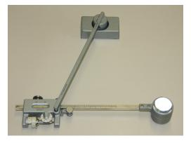
The planimeter consists of a two-bar linkage. At one end there is a pointer which is used to trace a closed curve, while the other arm allows the free movement of the device—though the base of the device remains fixed. The planimeter keeps track of the distance that a wheel fixed in place at the pointer rolls.<sup>2</sup> The planimeter then applies this information, using Vector Calculus, to display on an analog counter the total area enclosed by the curve.
