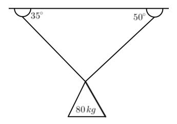
**26**. Find the tension in each wire in the diagram below.
