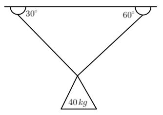
**25**. Find the tension in each wire in the diagram below.
